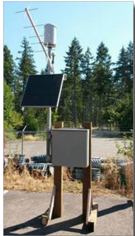
Working model of a rain gauge: Rain gauges provide an early warning when a deforested area is at risk for flash flooding. (rain gauge photo for Ecology's sf-299 application)
